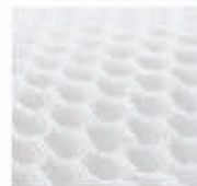
テラマック®が編み上げられた組織表面。この穴や起伏が植物の根を受けとめる。Holes and projections act as receptacles for roots. Structured surface knitted from TERRAMAC®. Holes and projections act as receptacles for roots.
